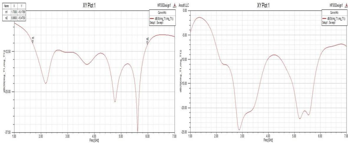
Fig.2  $S_{11}$  Vs Frequency curve when Both switches are ON Fig. 3  $S_{11}$  Vs Frequency curve when Left switch is ON
