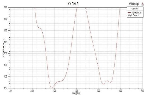
Fig. 8 VSWR when Left switch is ON
