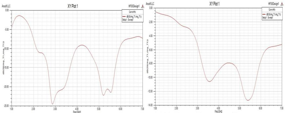
Fig. 4  $S_{11}$  Vs Frequency when Right switch is ON Fig. 5  $S_{11}$  Vs Frequency when Both switches are OFF
