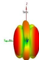
Fig. 11 Radiation Pattern when Left Switch ON
