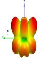
Fig. 10 Radiation Pattern when Both switches are OFF
