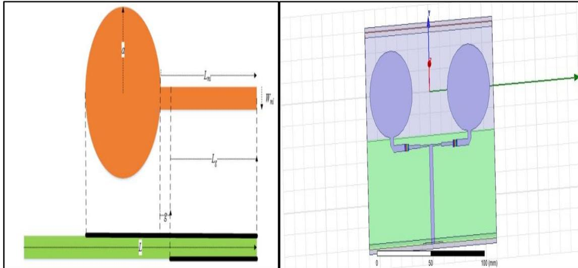
Fig. 1(a) Proposed Antenna Structure Fig. 1(b) Proposed Antenna Design
