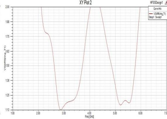
Fig. 9 VSWR when Right switch is ON
